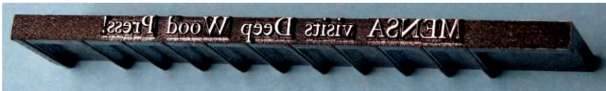
A slug of type produced by the Linotype machine.
