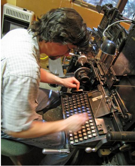
Chad Pastotnik quickly composes a line of type on his Mergenthaler Linotype machine - ca 1960.
